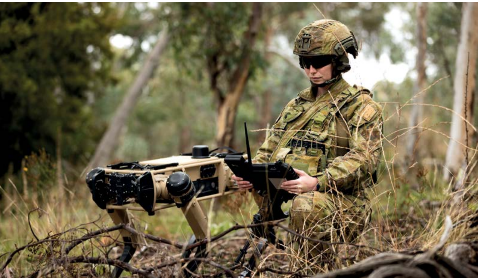
Australian Army soldier Corporal Meg Reeves uses a Ghost Robotics quadruped robot for a reconnaissance task at Mount Pleasant, Canberra.
