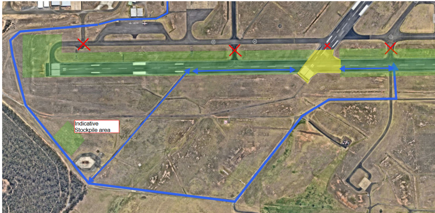
Figure 6 - Access Route for Intersection Asphalt Works
