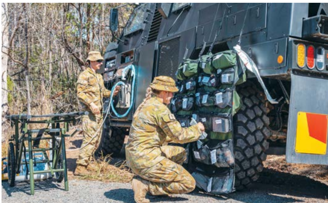
A Royal Australian Army Electric Protected Mobility Vehicle demonstrates the capability to provide power to enable a medical treatment team to deploy in the field at Gallipoli Barracks in Brisbane. IMAGE CREDIT: Corporal Nicole Dorrett.
