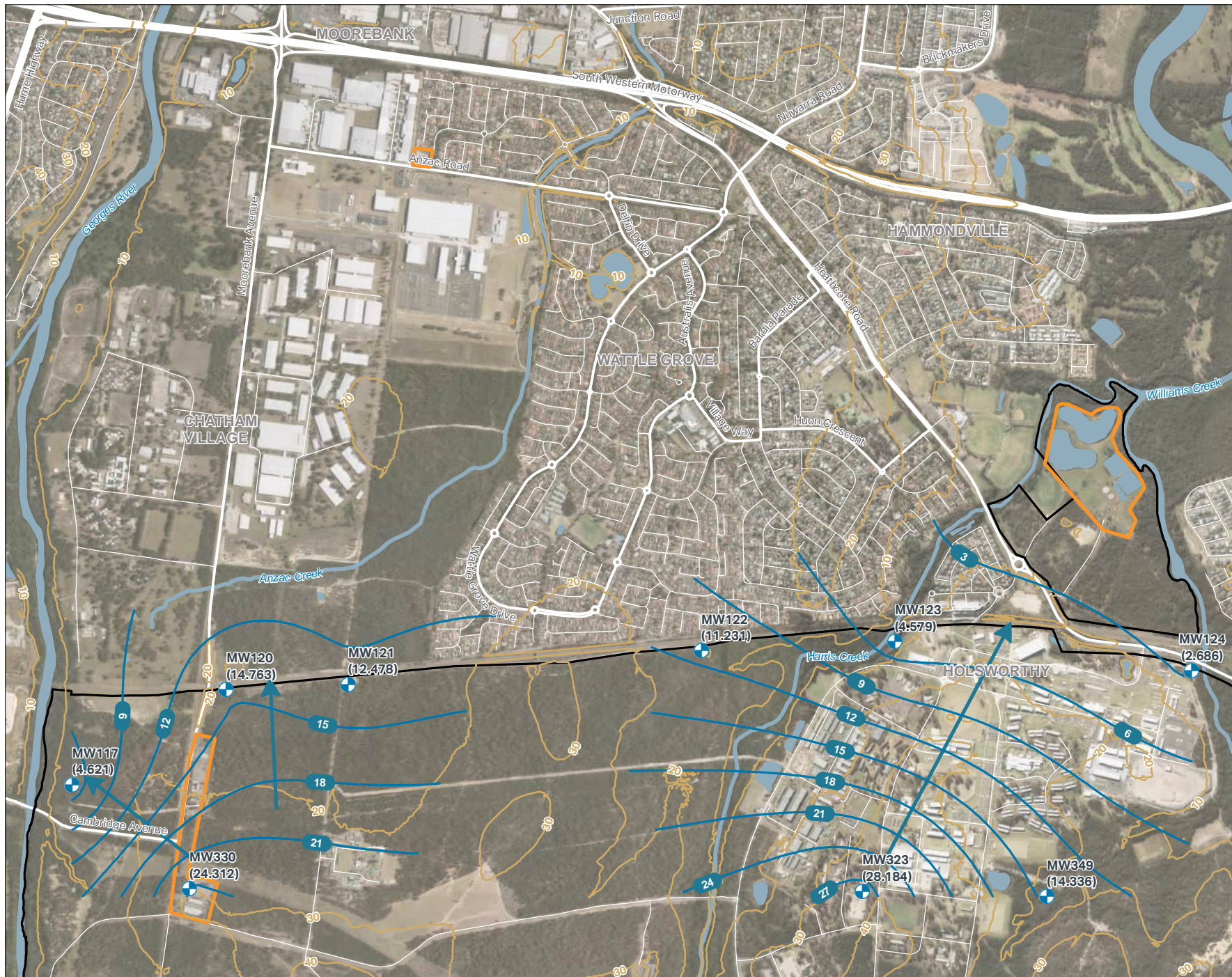
FIGURE F20-1: GROUNDWATER ELEVATION PLAN BEDROCK (MARCH 2023)
