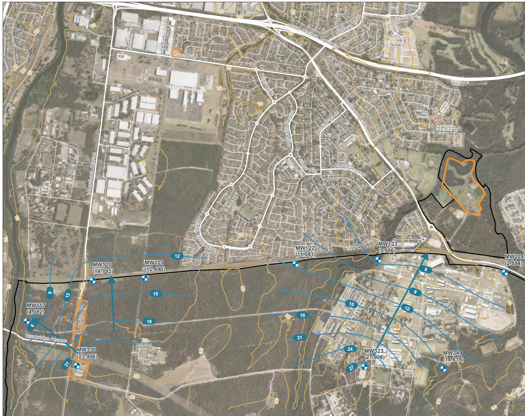
FIGURE F22-1: GROUNDWATER ELEVATION PLAN BEDROCK (SEPTEMBER 2022)
