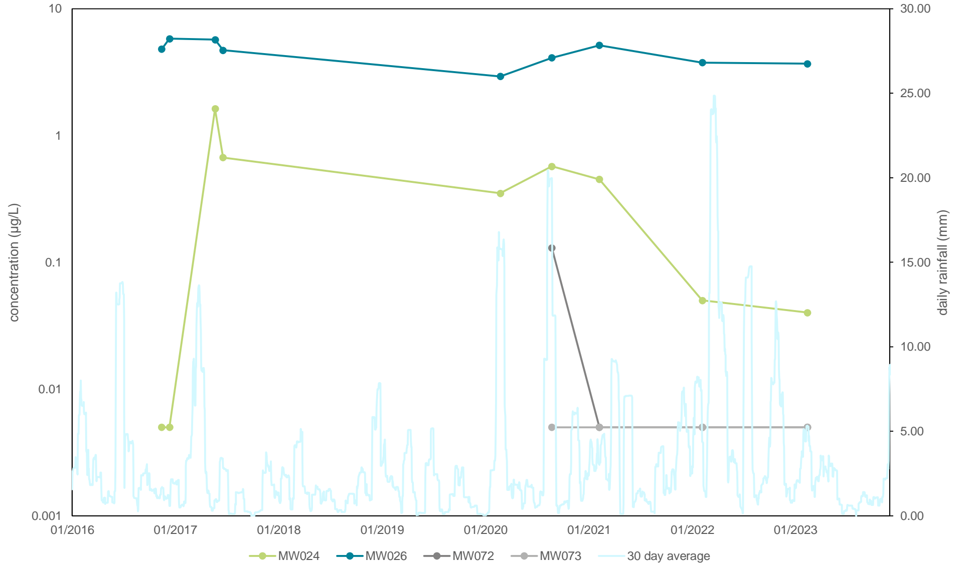
G10 - Temporal Trend Graph - Groundwater Off-Site locations (northwest and southeast of Site) - PFOS+PFHxS
