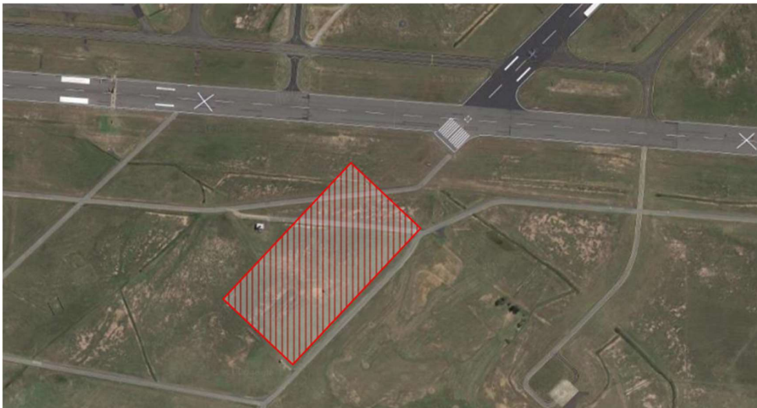
Figure 10 - Critical Area - Glide Path
