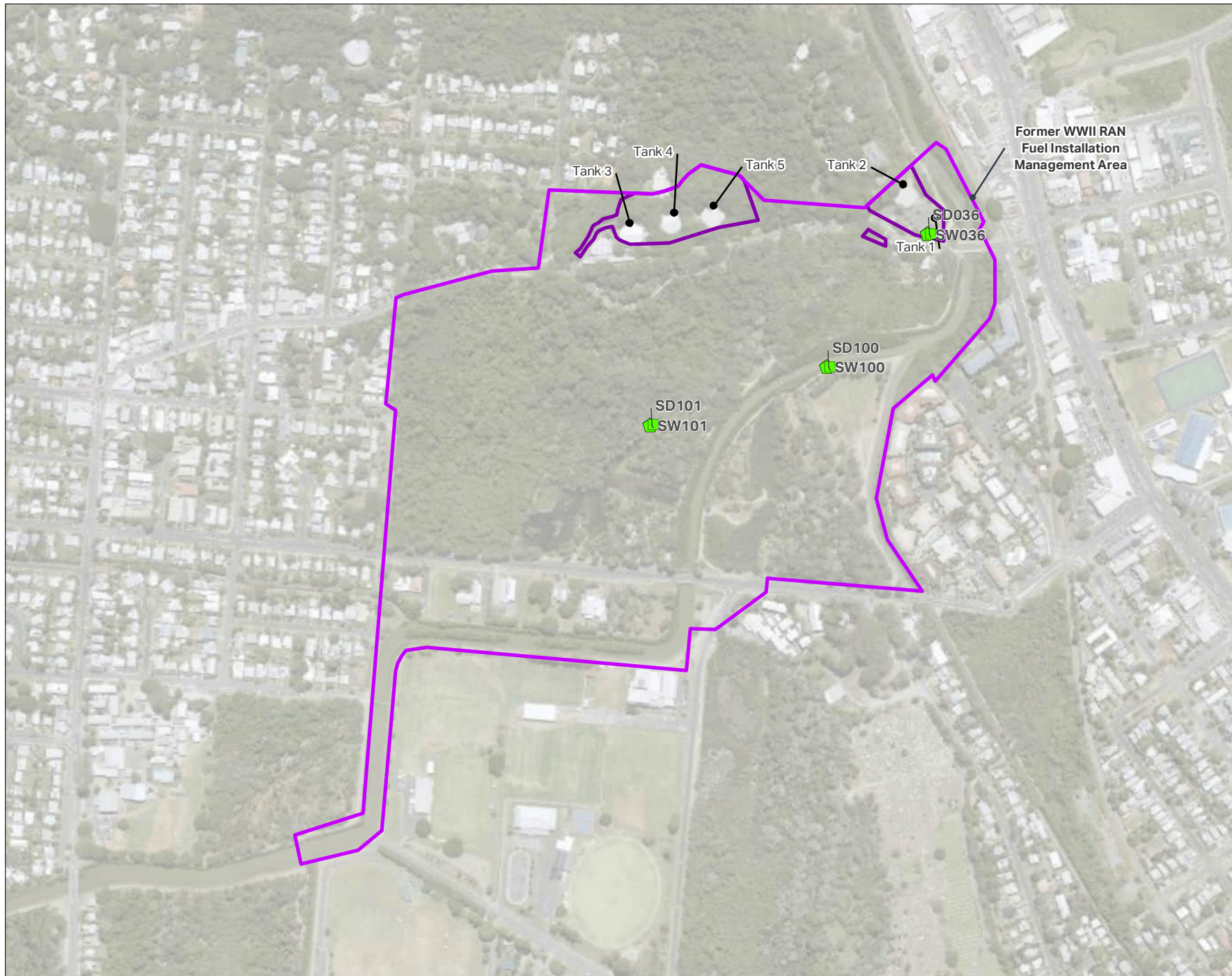
FIGURE F37: SURFACE WATER AND SEDIMENT RESULTS: WWII RAN FUEL INSTALLATION - PFOA (APRIL 2021)
