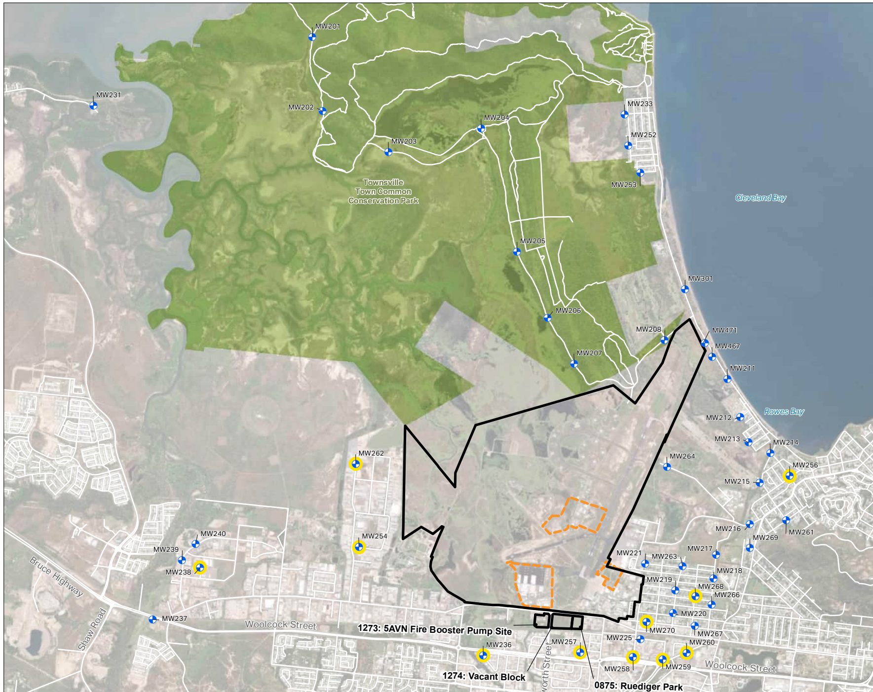
FIGURE 2b: OFF-BASE GROUNDWATER SAMPLING LOCATIONS
