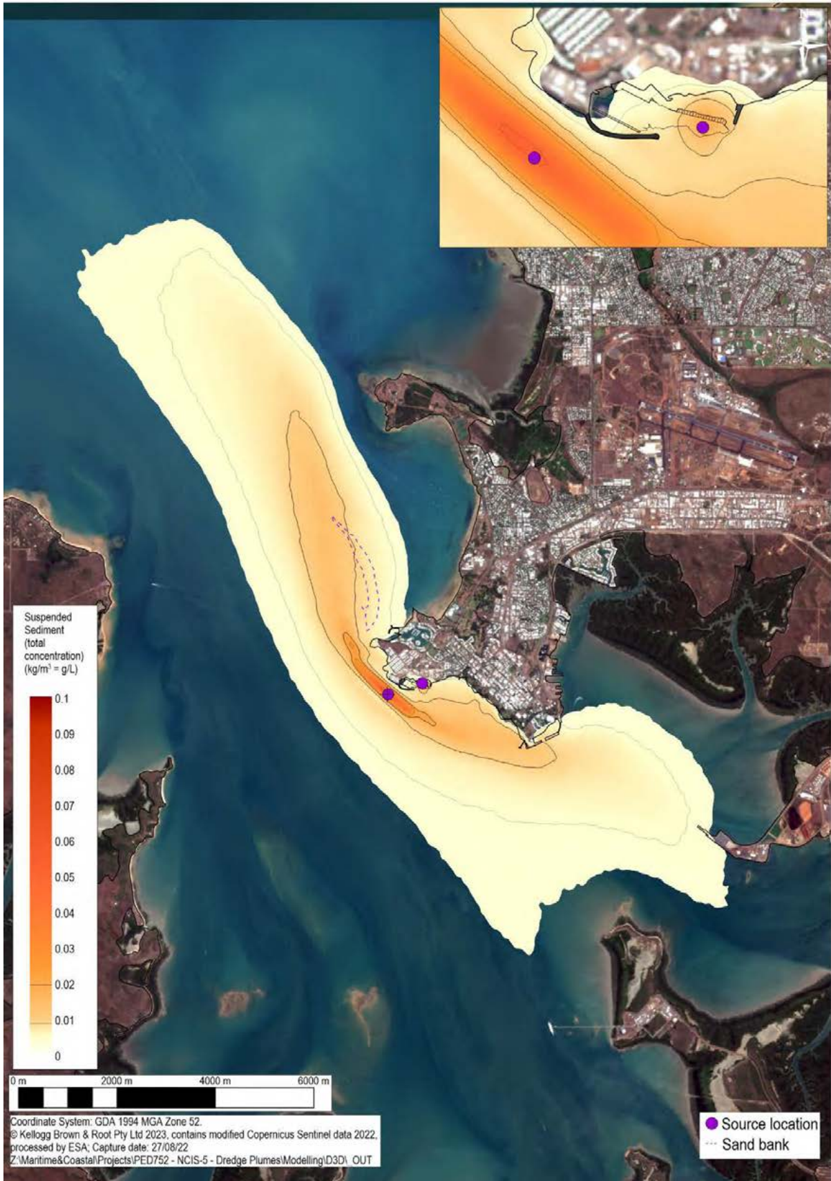
Figure 5.5 90 th Percentile suspended sediment concentration from CSD with offshore discharge – Dry season (includes 3 mg/L background concentration)
