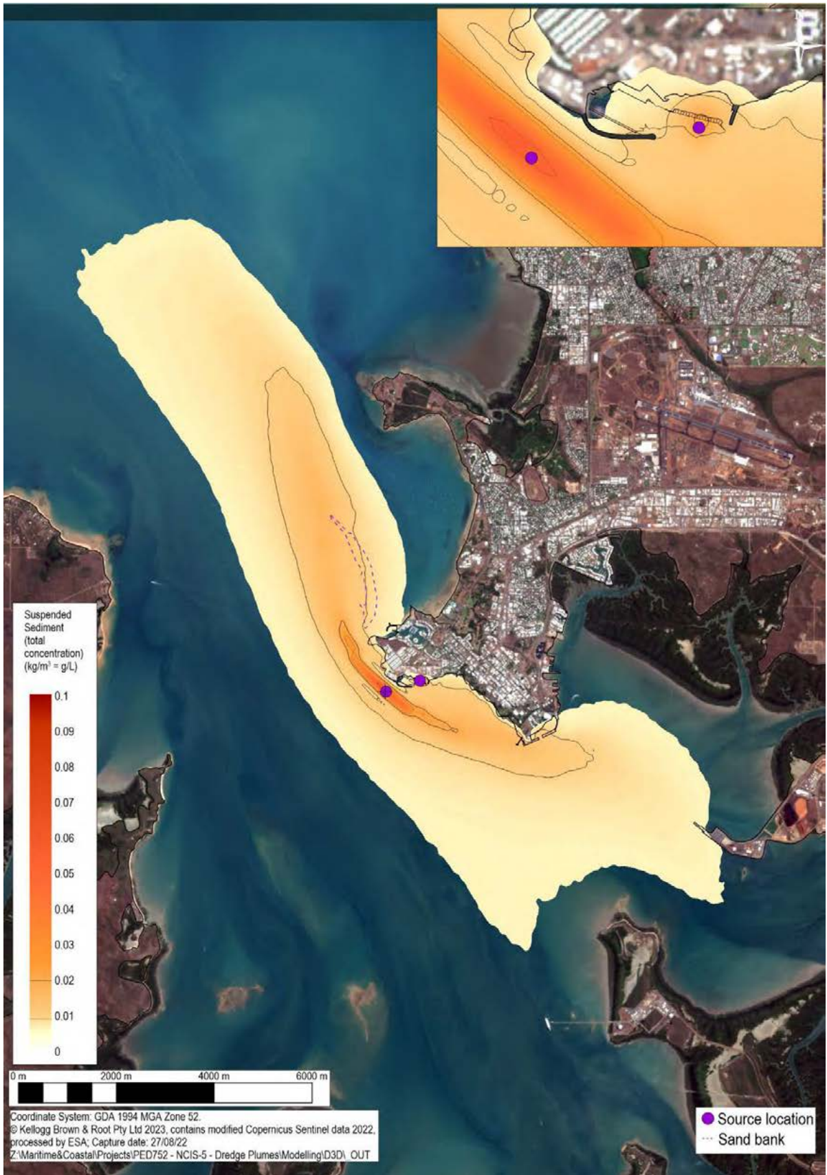
Figure 5.13 90 th Percentile suspended sediment concentration from CSD with nearshore discharge – Wet season (includes 5 mg/L background concentration)
