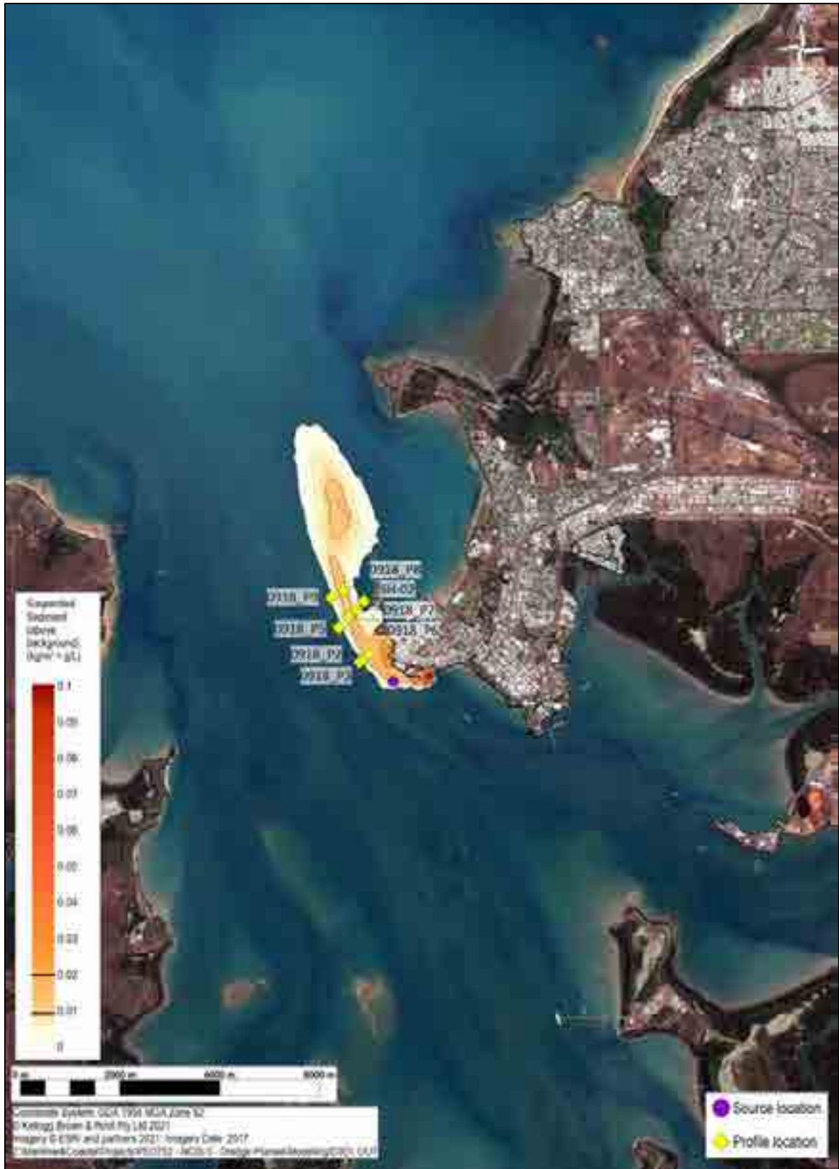
Figure 4.9 Suspended sediment concentrations above background – Depth-averaged instantaneous result with 18/9/13 monitoring locations
