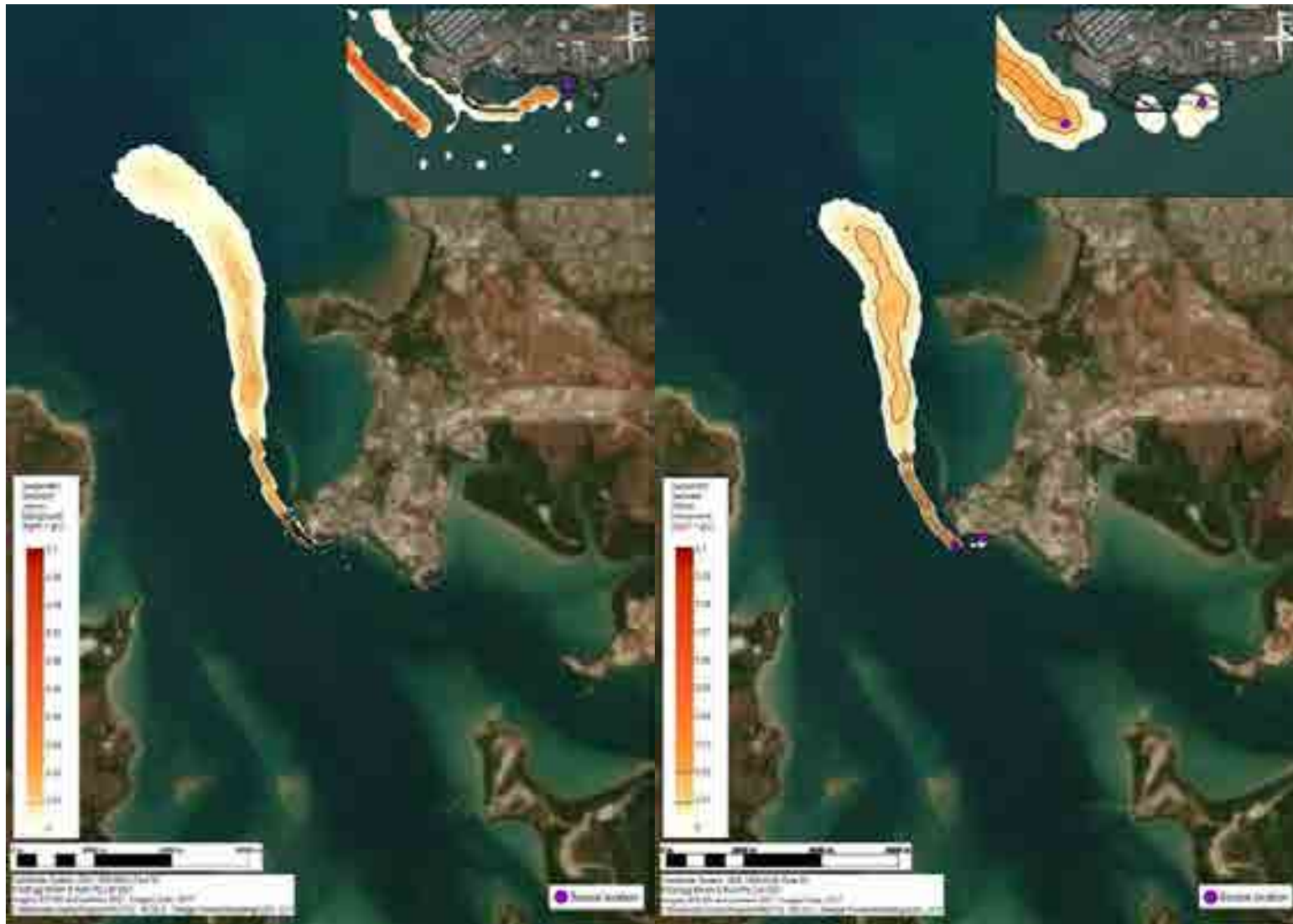
Figure C.4 Comparison of 2D (left) and 3D (right) modelled suspended sediment concentrations above background (depth-averaged) - Instantaneous result at 18/11/2017 13:00 – Ebb tide, spring condition
