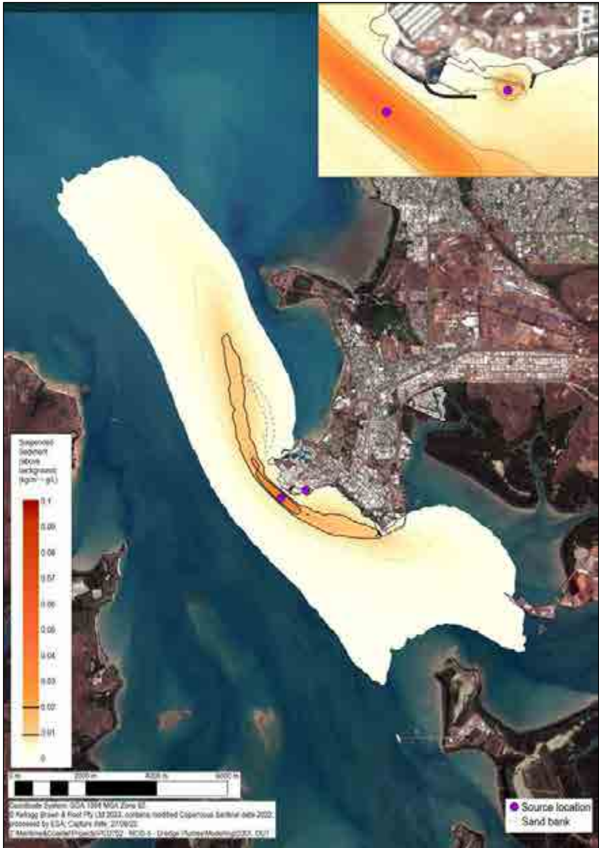
Figure 5.13 90 th Percentile suspended sediment concentrations above background - CSD dredging with nearshore discharge - NCIS-5 current works
