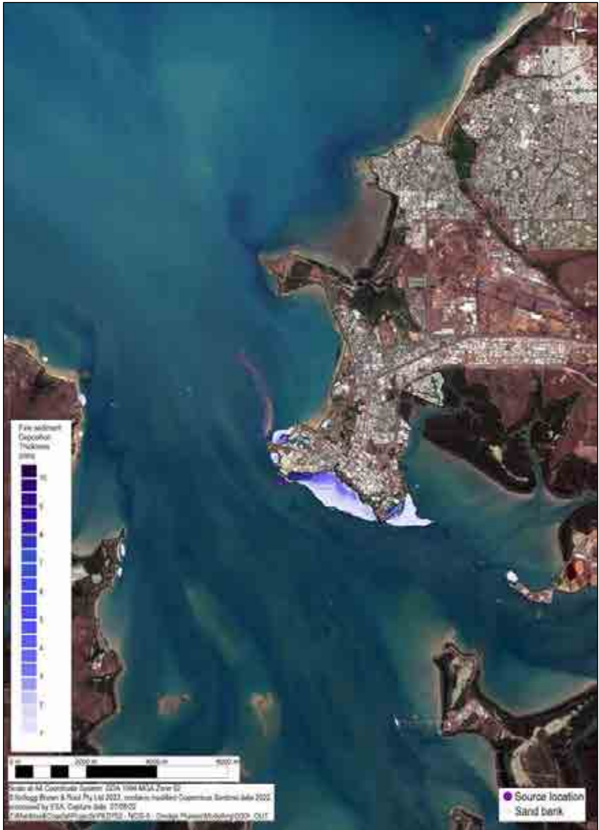
Figure 6.2 Zones of Fine Sediment Fate – Deposition thickness (mm) following dredging
