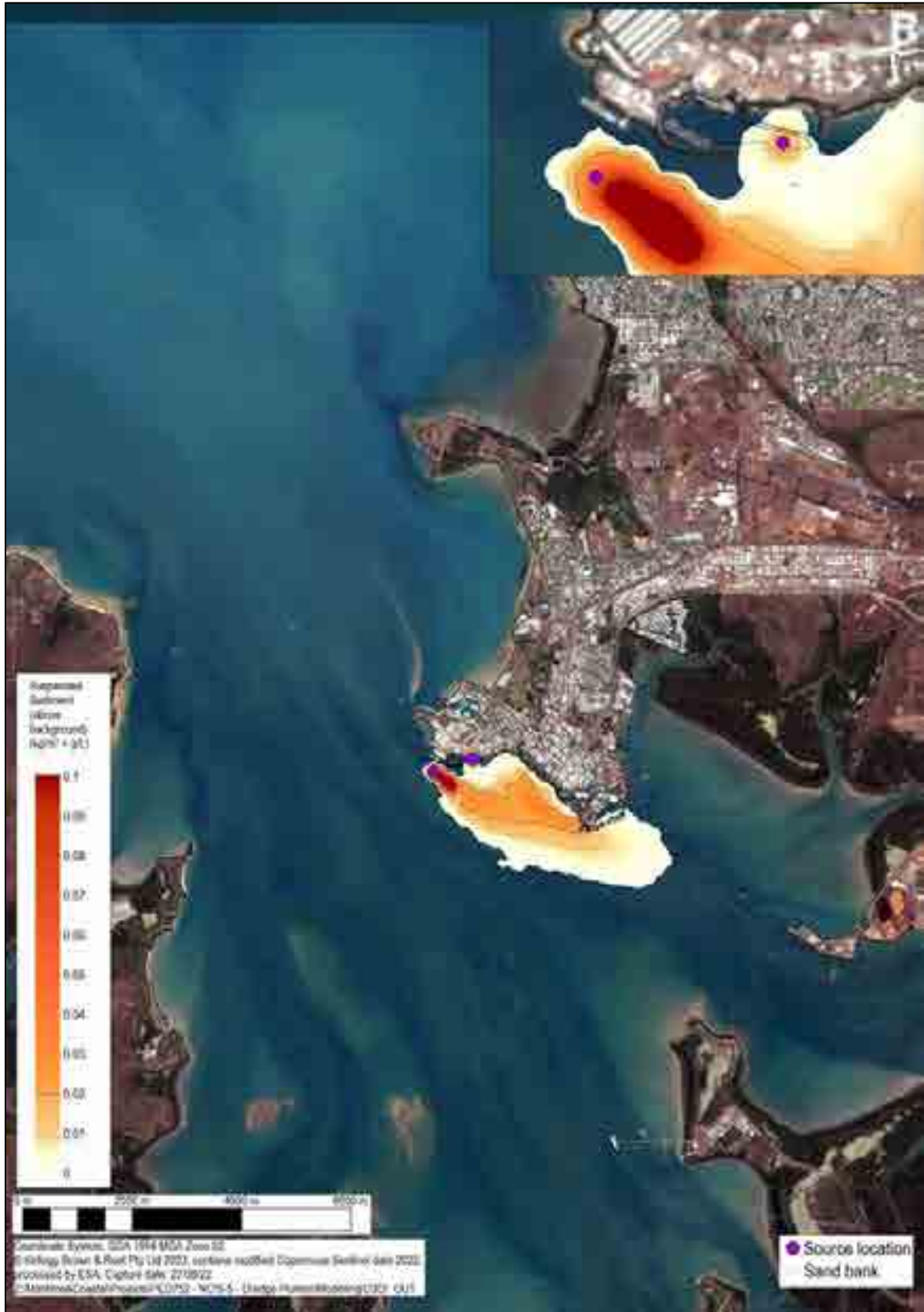
Figure 5.2 Suspended sediment concentrations above background - Instantaneous result at 12/11/2017 14:00 – Flood tide, neap condition
