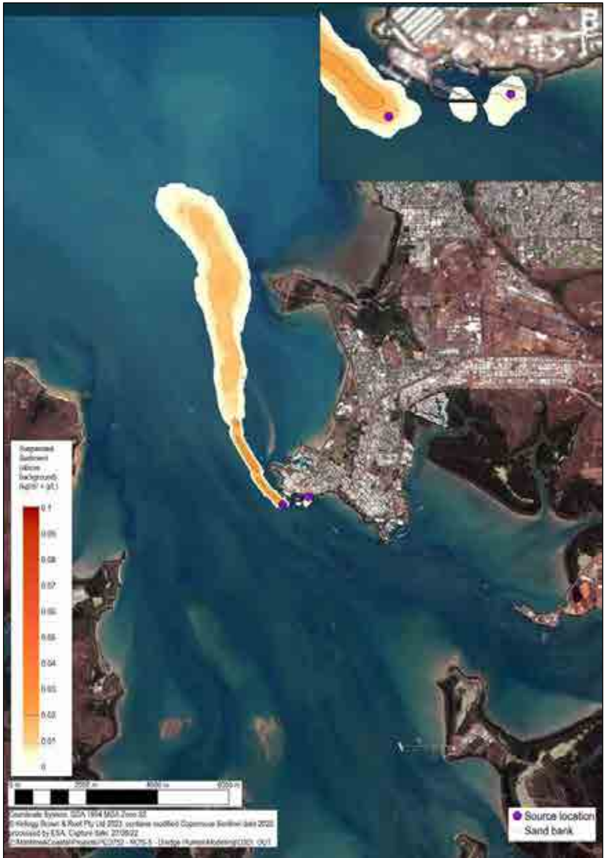
Figure 5.4 Suspended sediment concentrations above background - Instantaneous result at 18/11/2017 13:00 – Ebb tide, spring condition
