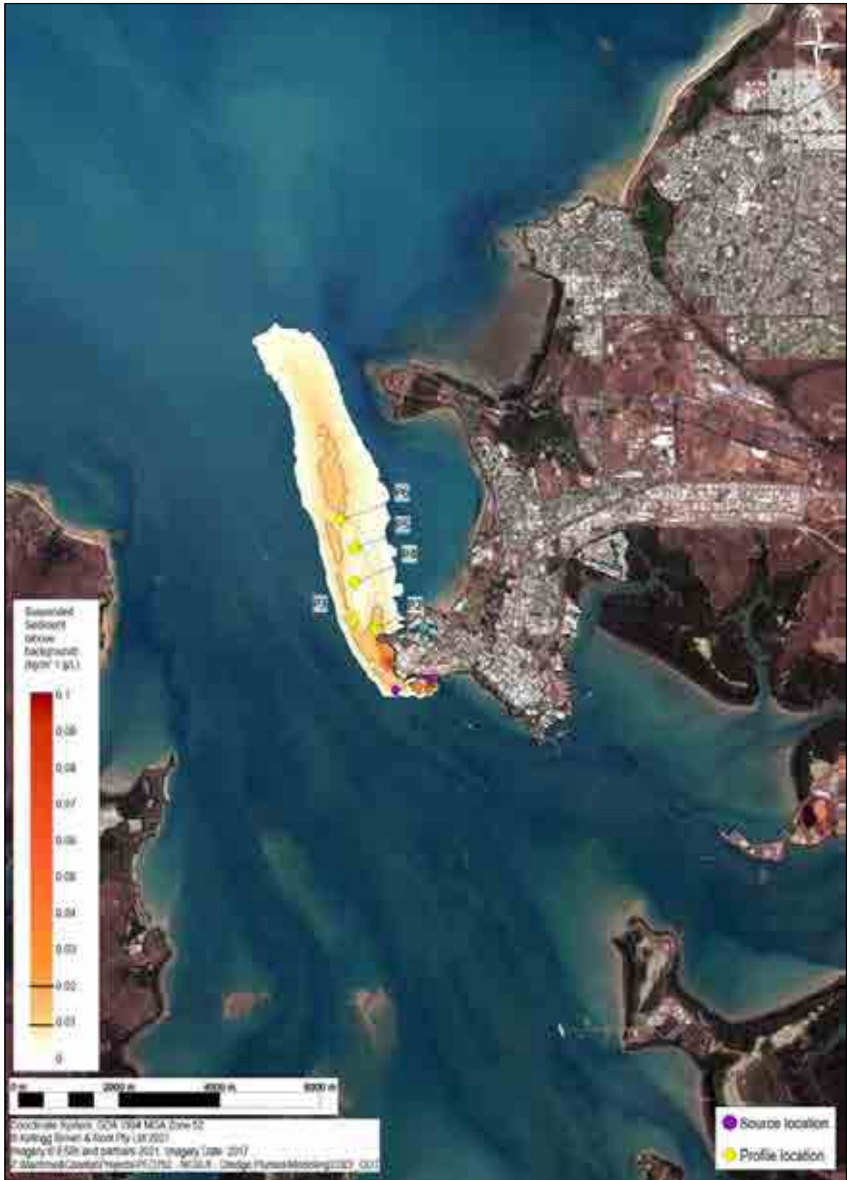
Figure 4.19 Turbidity monitoring sites at 13/07/2006 (compared to modelled plume extent)
