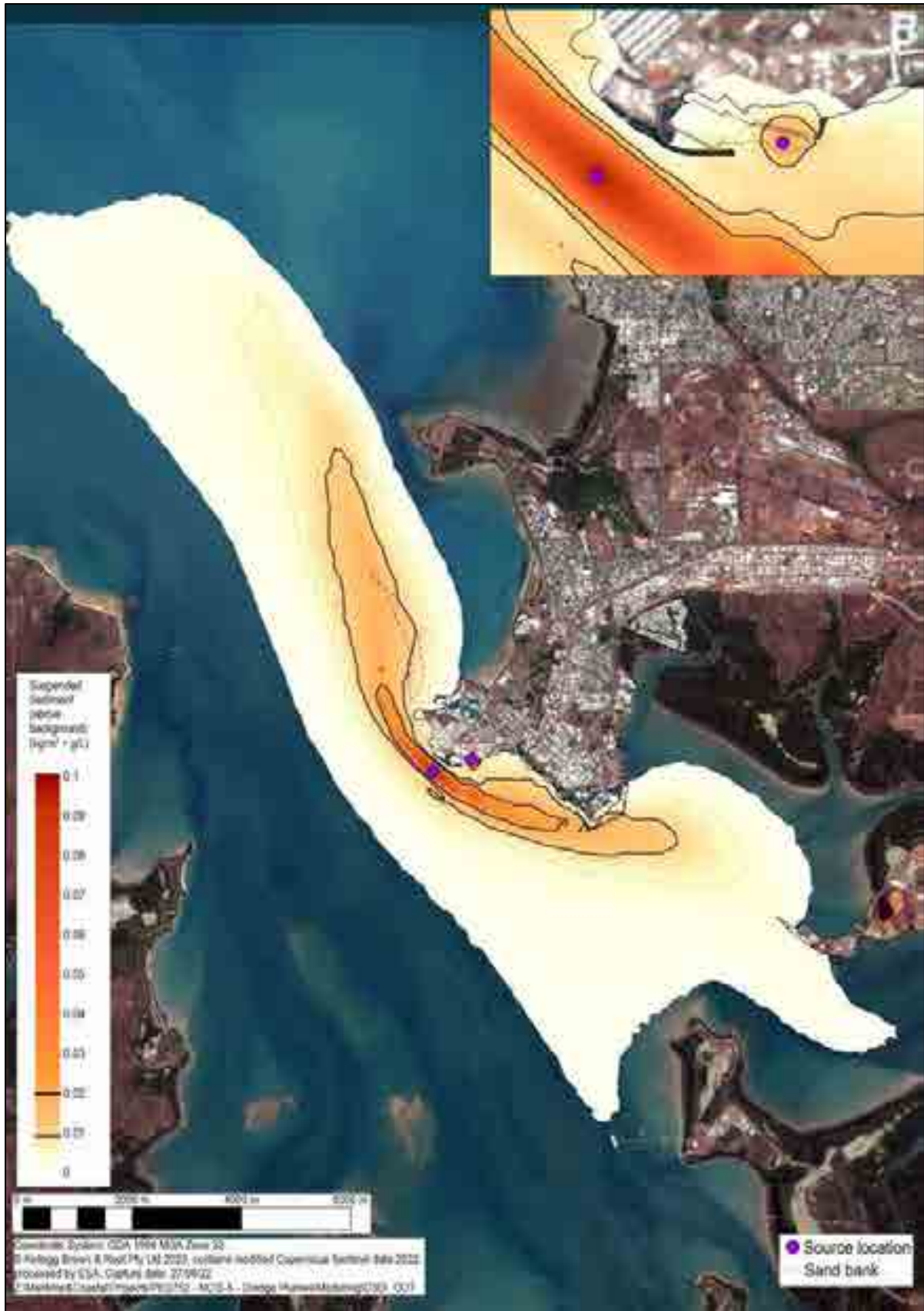
Figure 5.14 95 th Percentile suspended sediment concentrations above background - CSD dredging with nearshore discharge - NCIS-5 current works
