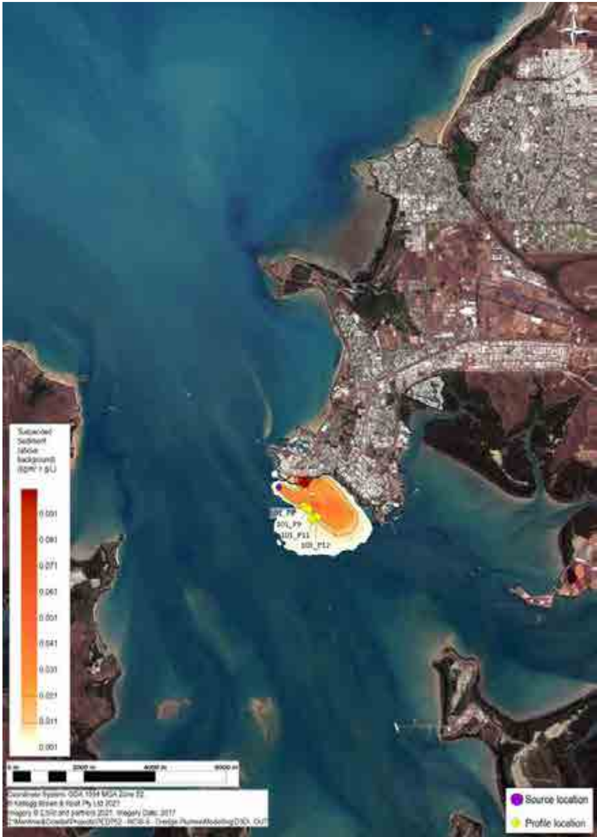
Figure B.5 Suspended sediment concentrations above background – Depth-averaged instantaneous result at 1/10/2013 08:30 with measured locations (with depth profile locations)
