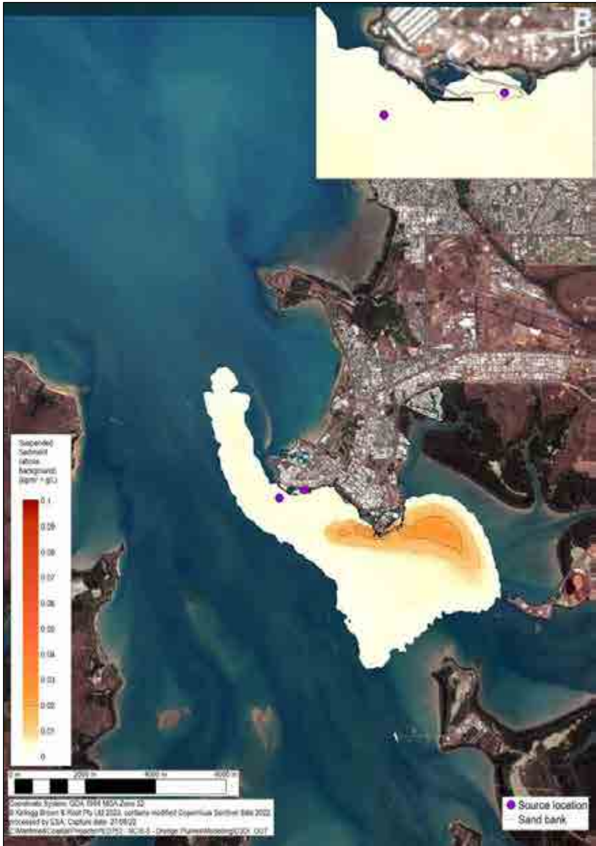
Figure 5.5 Suspended sediment concentrations above background - Instantaneous result at 18/11/2017 19:00 – Flood tide, spring condition
