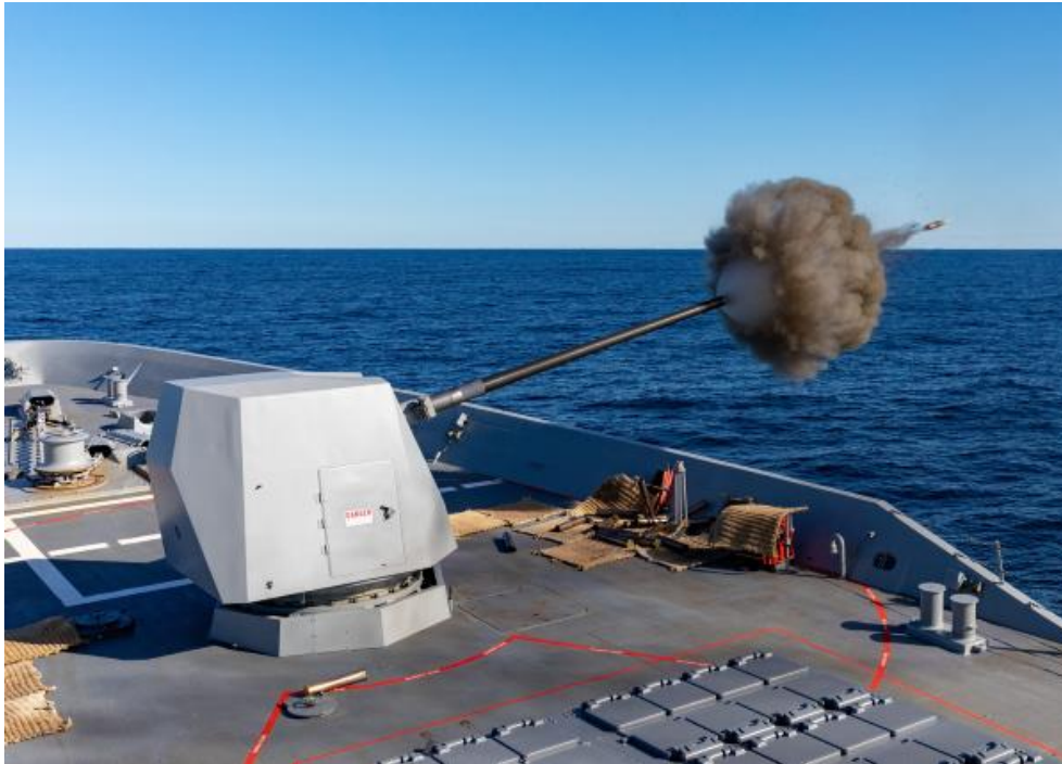
HMAS Hobart conducts a live fire exercise using the Mark 45 Mod 4 5-inch gun as a test of capability.
