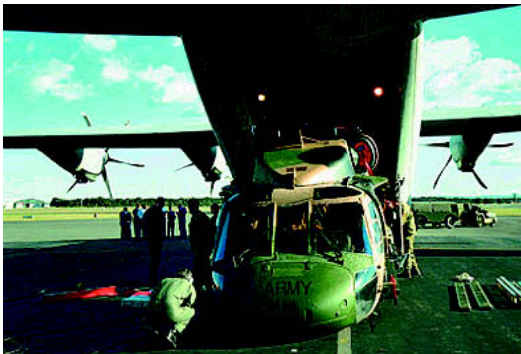
Army Blackhawk helicopter being loaded as cargo into a C130J model Hercules.
