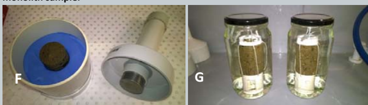
Photo C, D & E, Homogenised soil stockpiled - post mixing. Photo F, Typical equipment for the structural integrity procedure. Photo G, Typical leaching setup (LEAF Method 1315) which involves multiple leaching events of the undisturbed monolith sample.
